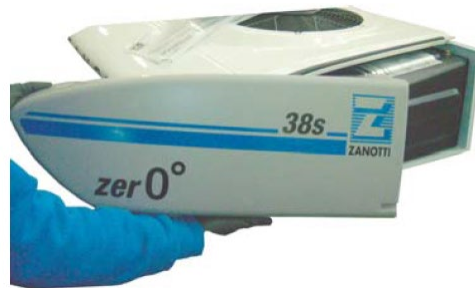
Figure 28 - Removing the side frame
