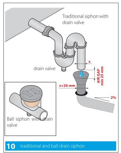
To avoid overflows from the collection tank, the siphon must have a **purge valve** that allows the removal of impurities deposited on the bottom.
