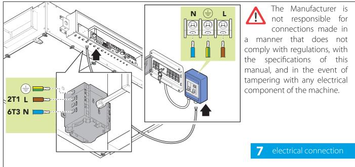
The actual supply voltage of the users **must not deviate more than 10%** from the normal voltage expected. Higher voltage differences cause damage to users and to the electrical system, malfunctioning of fans, noise. It is therefore essential to check the alignment of the actual voltage values with the nominal values.
